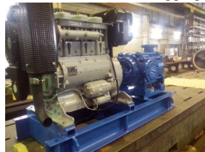
Diesel pomp units
